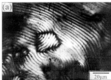
(5a) no anchoring, the width of the striations in the mesophase was about 2.6 \mu\text{m}
